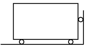
**Static equations must have 6 unknowns for 3space, or 3 unknowns for in-plane**  If you are not sure, then try solving for the reaction forces and moments.
