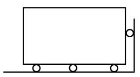
A body that is neither overconstrained nor underconstrained is called static determinant
