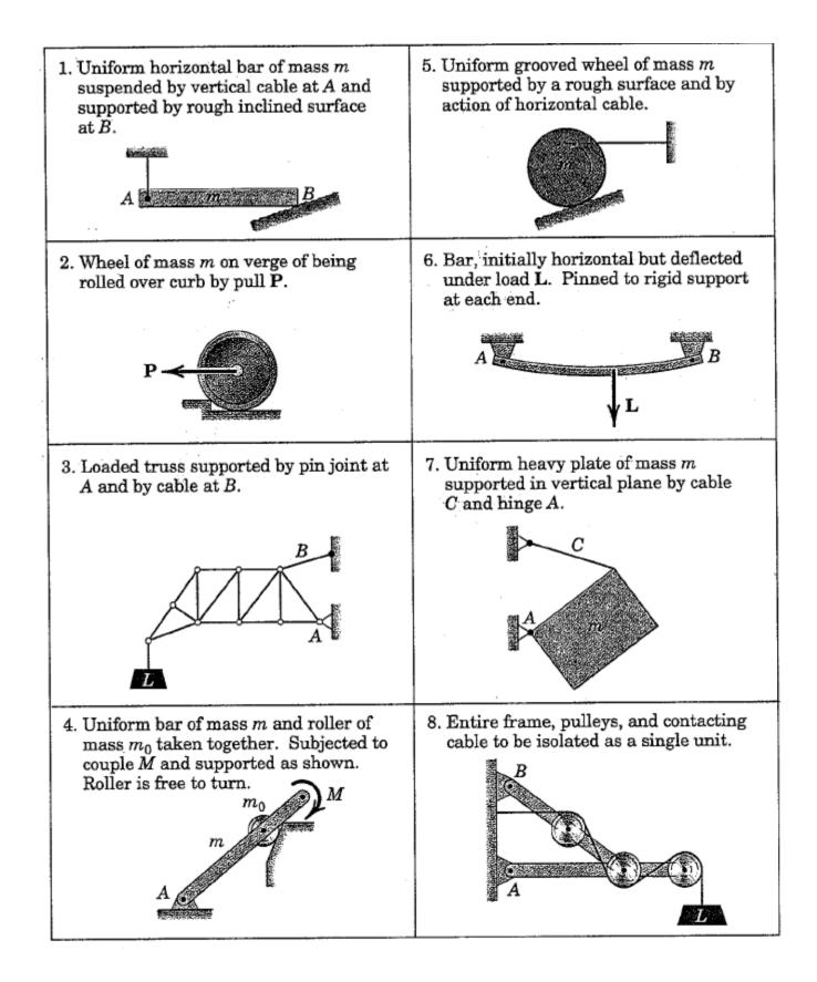
For a rigid body to be static, the net sum of forces and moments acting on it must be zero.
